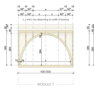
Structure: Timber Frames and Arches
