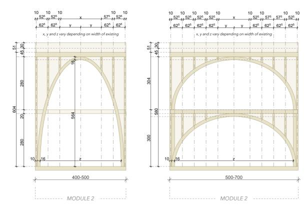
The main elements of the design are proposed as repetitive arches with framework in one or two story versions. However, the partition elements between flats for the larger models are composed of two arches on top of each other in order to allow for the support of the intermediate ceiling and to make the system more efficient.
